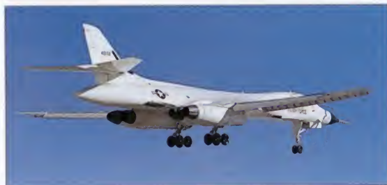
Below: The B-1A's undercarriage retracted into the fuselage between the engine nacelles. Each main leg was supported by a four-wheel bogie.
